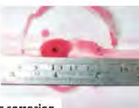
Found pitting corrosion
